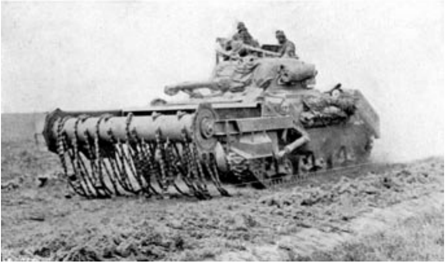
Tank rigged with flails to trigger mines
